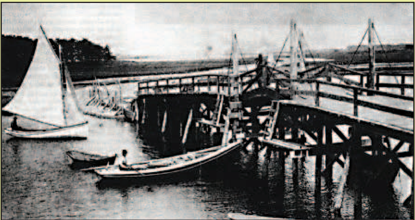
"Two Hamptons photographed around the turn of the century at Turbatis Creek in Kennebunkport, Me. Lance Lee of the Bath Marine Museum says that the boat at left is the only Hampton he has seen that was sloop rigged." John Gardner-The Small Boat Journal 1979
